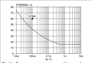
Fig.11. Damper maximum non-repetitive rms forward current.  $I_F = f(t_p)$ ; sinusoidal current waveform;  $T_j = 150$  °C prior to surge with reapplied  $V_{RWM}$ .
