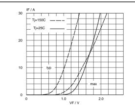
Fig.13. Damper forward characteristic  $I_F = f(V_F)$ ; parameter  $T_j$
