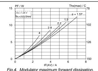
Fig.4. Modulator maximum forward dissipation,  $P_F = f(I_{F(AV)})$ ; sinusoidal current waveform; parameter  $a = form \ factor = I_{F(RMS)}/I_{F(AV)}$ .
