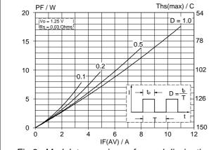
Fig.3. Modulator maximum forward dissipation,  $P_F = f(I_{F(AV)})$ ; square wave current waveform; parameter  $D = duty \ cycle = t_p/T$ .
