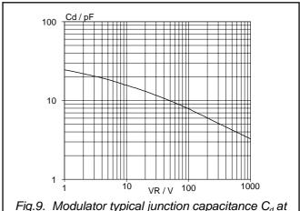
Fig.9. Modulator typical junction capacitance  $C_d$  at  $f = 1 \text{ MHz}_{,} T_{j} = 25 ^{\circ}\text{C}$
