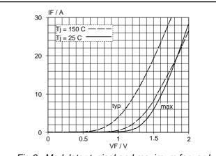
Fig.6. Modulator typical and maximum forward characteristic;  $I_F = f(V_F)$ ; parameter  $T_i$
