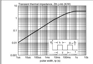
Fig. 12. Damper transient thermal impedance  $Z_{th} = f(t_p)$
