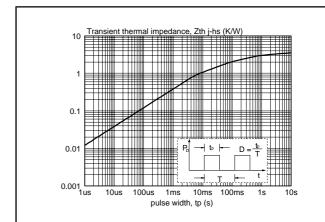
Fig.10. Modulator transient thermal impedance  $Z_{th} = f(t_p)$
