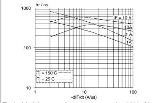
Fig.8. Modulator maximum  $t_{rr}$  measured to 25% of  $I_{rmr}$ ;  $T_j = 25^{\circ}\text{C}$  and 150  $^{\circ}\text{C}$
