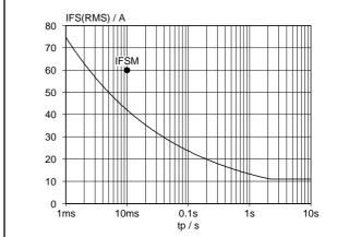
Fig.5. Modulator maximum non-repetitive rms forward current.  $I_F = f(t_p)$ ; sinusoidal current waveform;  $T_j = 150$  °C prior to surge with reapplied  $V_{RWM}$ .
